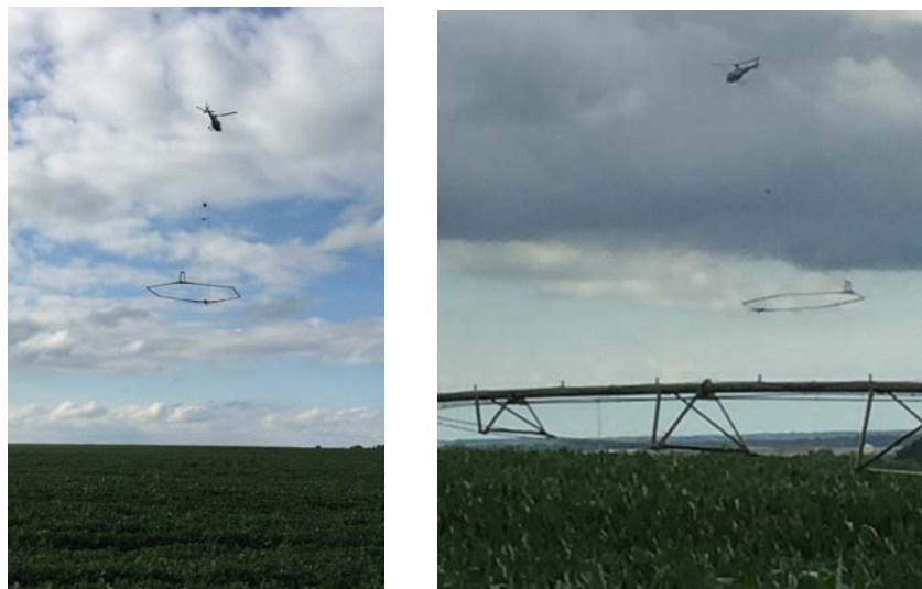
Figure 2-4. Photos of the SkyTEM304M system in suspension beneath the helicopter.
